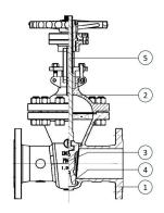
Stellite-reinforced sealing between seat and wedge.
