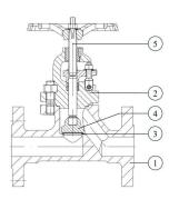
Stellite-reinforced sealing between seat and globe.
