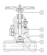
Stellite-reinforced sealing between seat and globe
