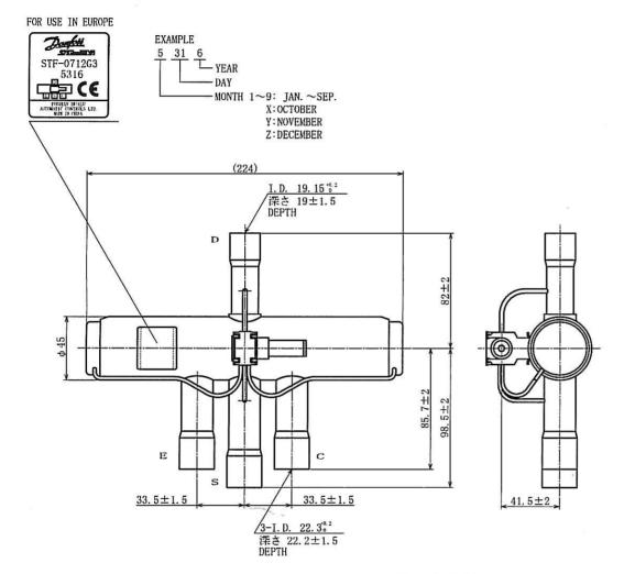
CONNECTIONS INDICATED BELOW SHOW AT COOLING MODE (WHEN COIL IS DE-ENERGIZED)
