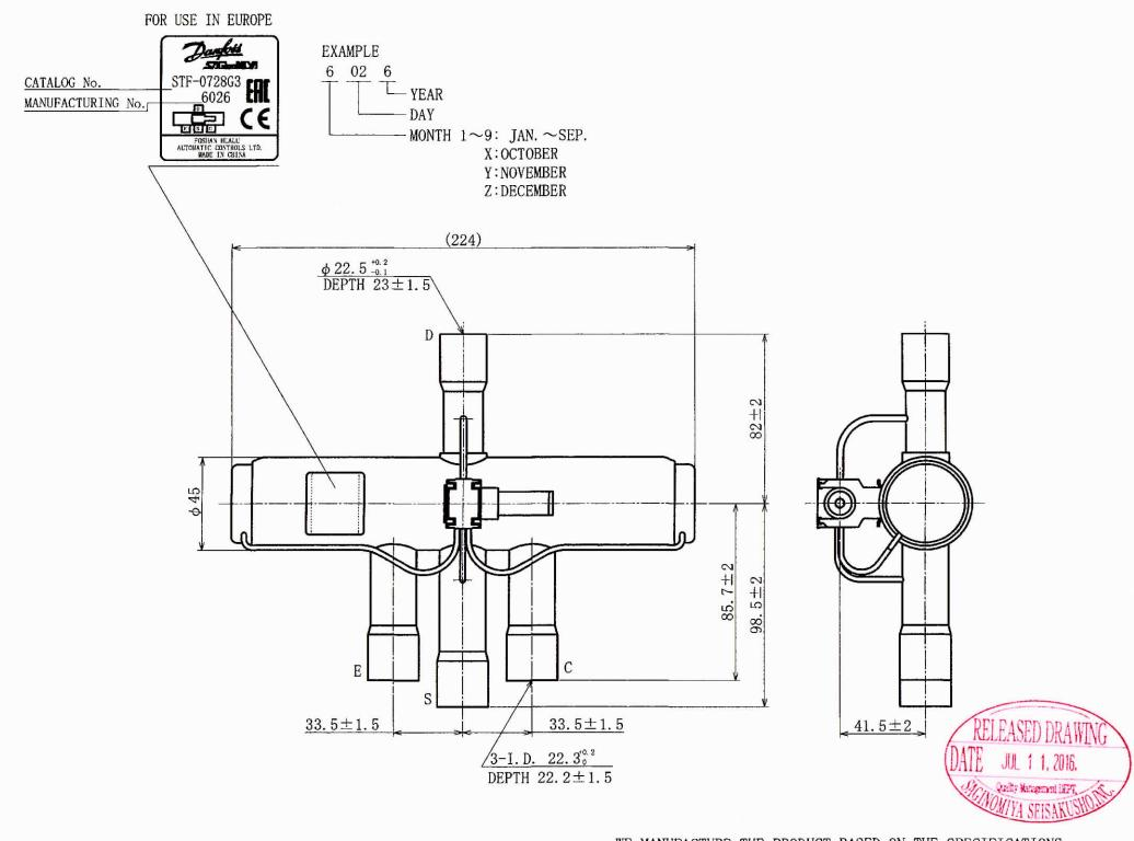
CONNECTIONS INDICATED BELOW SHOW AT COOLING MODE (WHEN COIL IS DE-ENERGIZED)
