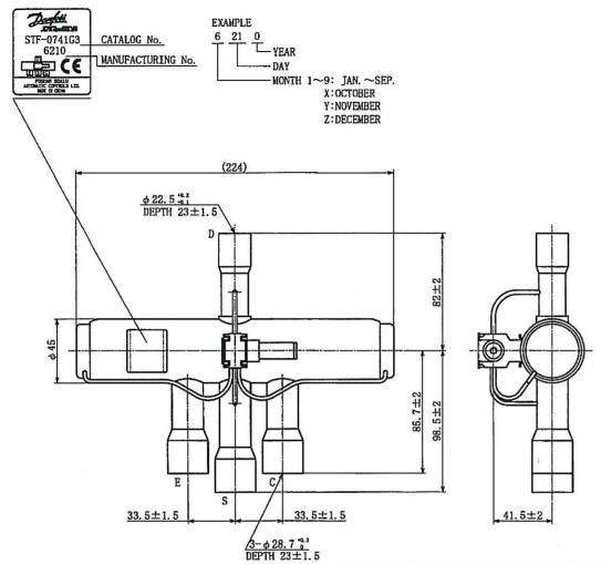
CONNECTIONS INDICATED BELOW SHOW AT COOLING MODE (WHEN COIL IS DE-ENERGIZED)
