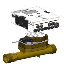
Subsequently fix the calculator on the plastic part with the help of the DIN mounting clip of the calculator
