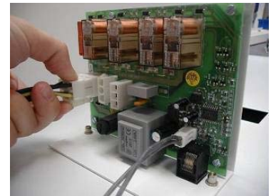
Unplug the two connectors of plate pressing the fluke.
