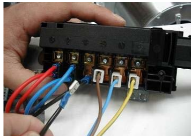
Unplug the cables to 1, 2, 3 in the connection box.
