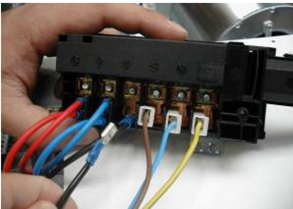
Unplug cables 1,2,3 of the junction box
