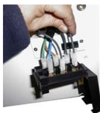
Disconnect the cables 2, 3, 4 of the connections box.
