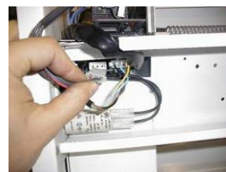
Disconnect the two connectors from the PCB board (J7 and B3).
